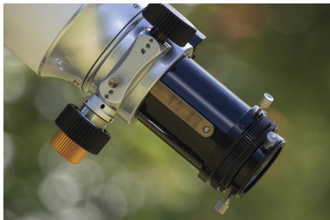
▲ Helical rack-and-pinion gears drive the focus movement and could support all the author's heavy imaging gear even when aimed toward the zenith. The 2-inch adapter uses a compression ring to ensure a solid purchase on accessories, though it may inadvertently tip some in the optical path (see the accompanying text for details). Threaded holes on the underside of the focuser allowed for easy installation of a ZWO EAF focus motor bracket.
