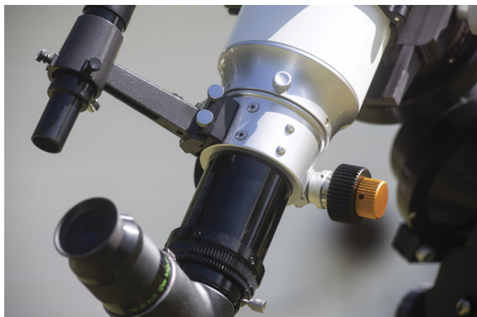
▲ The focuser has a 2.5-inch-aperture drawtube with 90 mm of travel and a printed scale on the outside. Its dual-speed focuser includes two course-adjustment knobs and one gold anodized, 10× reduction fine-focus knob. A 2-inch adapter threads into the end of the drawtube with 63-mm threads. Although a finder isn't included, the scope has a mounting base that accepts universal finder brackets. The entire focuser is rotated by loosening the silver thumbscrew and turning the unit.
