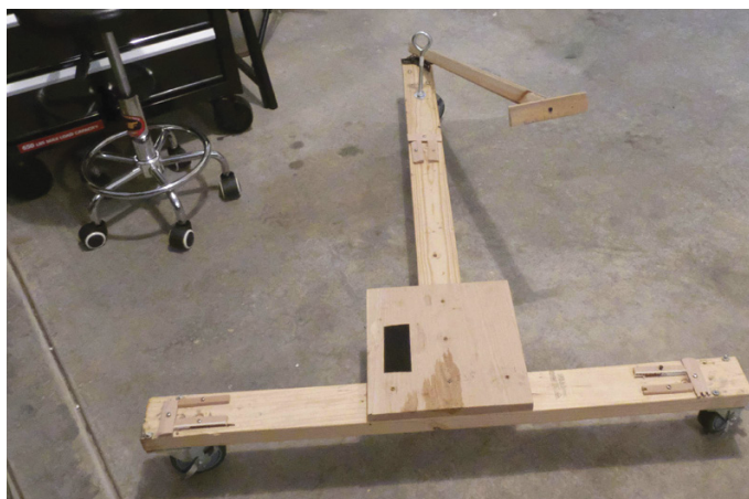
▲ Left: Peter's first attempt at a scope dolly was shaky and too low to the ground. Right: The second iteration with larger wheels was an improvement, but still not ideal.
