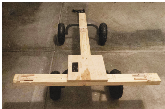
▲ Left: Peter's first attempt at a scope dolly was shaky and too low to the ground. Right: The second iteration with larger wheels was an improvement, but still not ideal.
