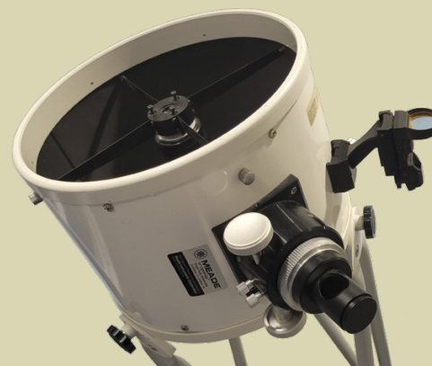
▲ SCOPES AND SIGHTS Top: Not so long ago, every telescope came with a finder-scope, like the Meade ETX125 seen at top, with a 24-mm right-angle finder conveniently located to the right of the main scope's eyepiece. Above: Most commercial telescopes today come equipped with a reflex sight.
