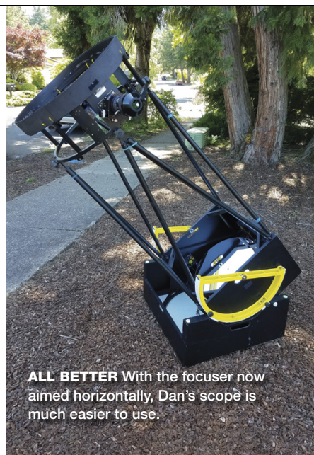
▲ TURN THE CAGE Rotating the secondary cage on a truss Dob is simple. You might have to make new mounting brackets, but that’s what angle iron is for. Note the original factory mounting point farther back to the right.
