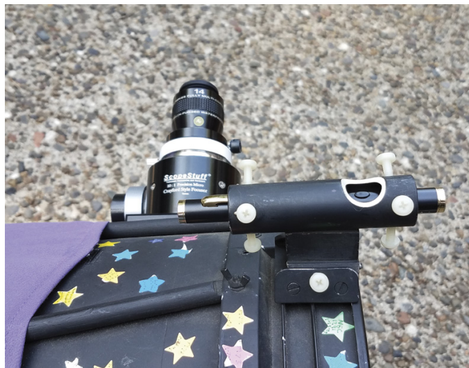
▲ LASER-GUIDED A green laser pointer makes a dandy finder. See my column on making the mount in the March 2022 issue, page 72.
