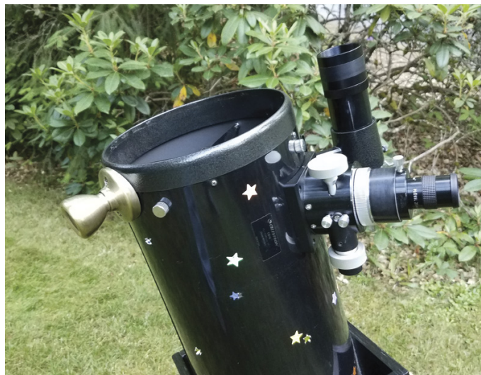
▲ GRIPPING CONVENIENCE A hand knob helps you move the telescope smoothly. Yes, that's a doorknob. They're made for hands.
