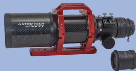
▲ The telescope comes with red anodized tube rings, a 245-mm-long Vixen-standard dovetail bar, and a top handle. A 2-inch visual back with 1 1/4-inch adapter is standard, but the 0.8× Reducer/Field Flatteners shown is a $200 option.
