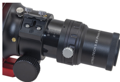
▲ Left: The locking knobs for the focuser (left) and the camera angle adjuster (right) are large and easy to use with gloves on. The Reducer/Field Flatteners has 48-mm threads on the camera side. Right: For balancing heavy cameras, the dovetail bar can be reversed to extend back another 60 mm from the position shown. The focuser is compatible with most focus motors.
