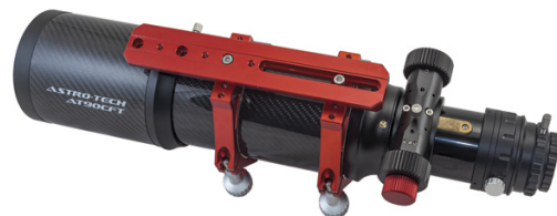
▲ Left: The locking knobs for the focuser (left) and the camera angle adjuster (right) are large and easy to use with gloves on. The Reducer/Field Flatteners has 48-mm threads on the camera side. Right: For balancing heavy cameras, the dovetail bar can be reversed to extend back another 60 mm from the position shown. The focuser is compatible with most focus motors.
