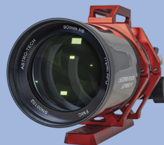
▲ The 90-mm triplet objective is fully multi-coated, and the tube interior is well-blackened and fitted with two mid-tube baffles to suppress stray light. The focuser is also ribbed with a series of knife-edge baffles.
