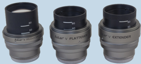
▲ The three included flatteners can each be configured to operate with either the 60-mm or 80-mm objectives by sliding their internal barrels between two locking positions. All are shown in their extended 60-mm settings.
