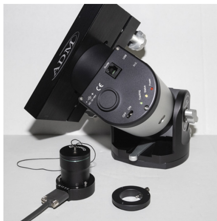
▲ Left: Users with a QHYCCD PoleMaster or similar polar-alignment aid can connect the included adapter to the raised disk on the north-facing end of the polar axis. Right: After securing the adapter, you can then quickly connect or remove the PoleMaster camera after use.
