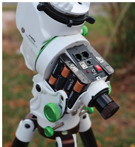
▼ The Star Adventurer GTi can be powered with 8 AA batteries. The batteries will power the mount in the event of failure from an external power supply.
