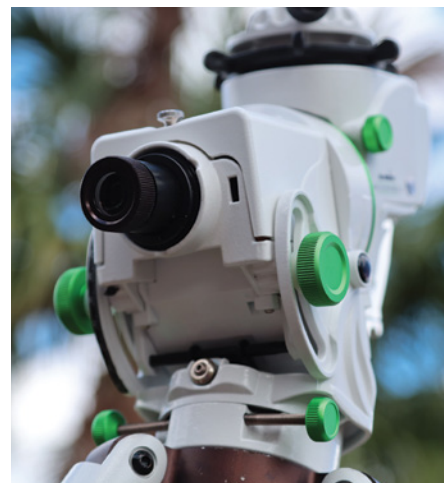
▼ The rear of the right-ascension axis contains the polar-alignment scope. A black plastic cover protects the polar scope's eyepiece when not in use.
