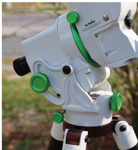
▼ The mount can operate between 0° and 70° latitude. Knurled green knobs on the azimuth and altitude controls are used during polar alignment. The right ascension clutch knob is visible at top.
