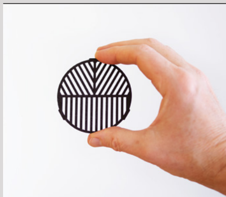
▲ MASKING FOR FOCUS Left: The author uses this Bahtinov mask from Farpoint Astro with his 300-mm telephoto lens. The mask installs much like a standard lens filter and allows for precise focusing. Right: This pair of images illustrates how to focus a lens fitted with a Bahtinov mask. When the central diffraction spike is positioned exactly halfway between the two diagonal spikes (far right image), the lens is perfectly focused.
