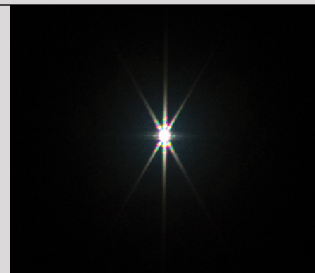
▲ MASKING FOR FOCUS Left: The author uses this Bahtinov mask from Farpoint Astro with his 300-mm telephoto lens. The mask installs much like a standard lens filter and allows for precise focusing. Right: This pair of images illustrates how to focus a lens fitted with a Bahtinov mask. When the central diffraction spike is positioned exactly halfway between the two diagonal spikes (far right image), the lens is perfectly focused.
