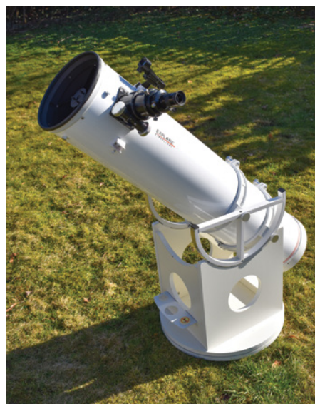
▲ STORE-BOUGHT GOODS Modern, commercially manufactured Dobsonians, like this 8-inch model from Explore Scientific, usually deviate from John Dobson's design, but the best examples retain the original's stability and ease-of-use.
