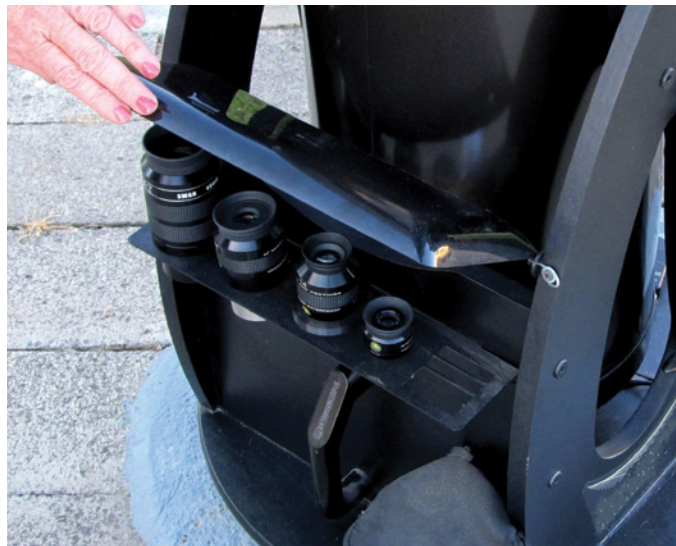
▲ Left: A simple cover over the eyepieces prevents dew from forming on them. Right: The cover lifts up to allow access to the eyepieces.
