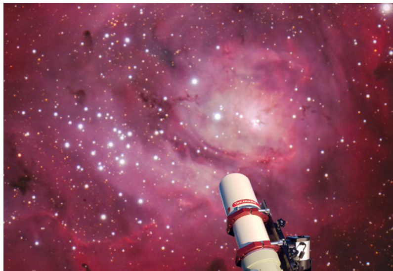
▲ HIGH-END ASSIST Astrophotographer John Gleason assembled his own electronically assisted astronomy setup to take high-quality, live-stacked images. He combined a Rainbow Astro RST-150 robotic mount with a Takahashi FSQ-106ED astrograph with a QHY5III-462C color camera. These images of M20 (left) and M20 (right) total 9 minutes each using SharpCap in Livestack mode. Gleason then processed the images in Adobe Photoshop .
