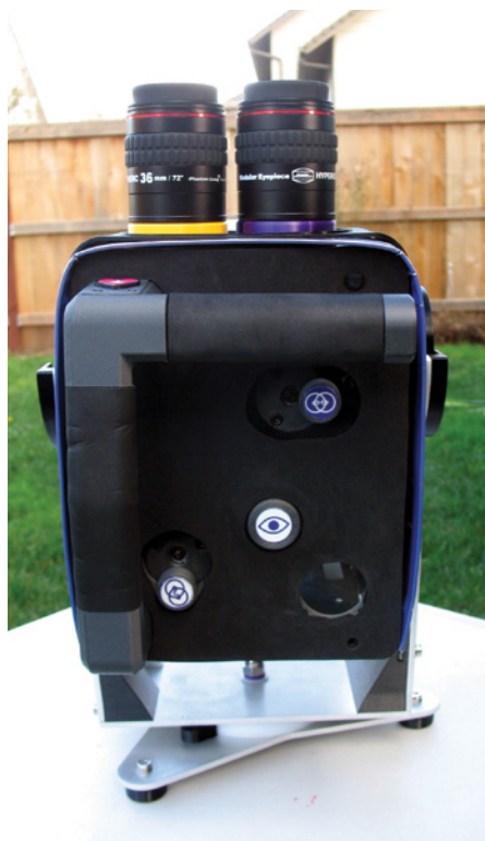
▲ The controls for image merging and interpupillary distance are easily accessible on the back of Robert's binoscope.
