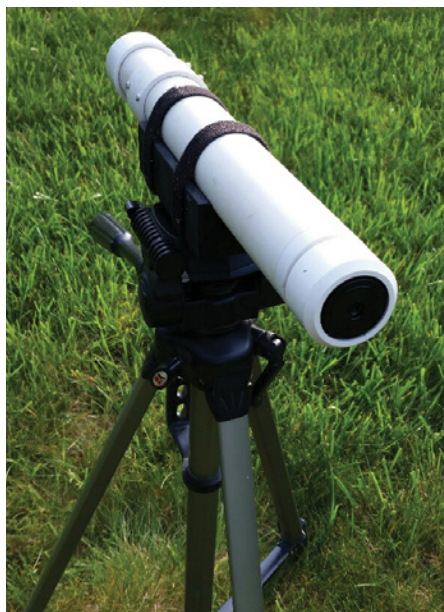
▲ Left: The eyepiece end of John's artificial star faces the telescope. In theory, the eye lens should face the light source and the field lens should face the telescope, but with a Plössl eyepiece's symmetrical design, it doesn't matter. Right: John designed his artificial star to have two brightness levels.
