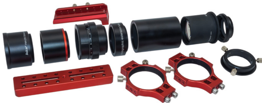
▲ All the FMA230's parts can unscrew from each other. The metal dew cap extends 50 mm (2 inches) and is threaded to accept 58-mm photographic filters.
