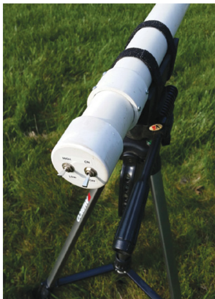
▲ Left: The eyepiece end of John's artificial star faces the telescope. In theory, the eye lens should face the light source and the field lens should face the telescope, but with a Plössl eyepiece's symmetrical design, it doesn't matter. Right: John designed his artificial star to have two brightness levels.
