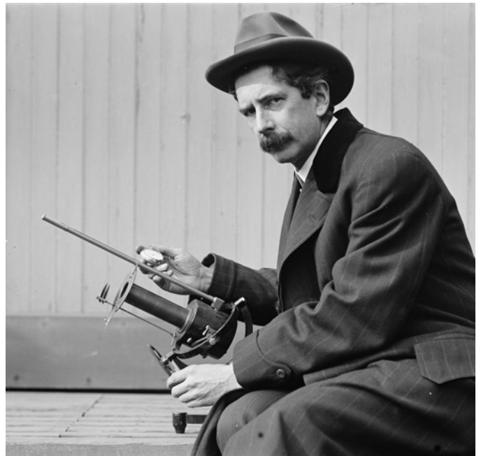
▲ SOLAR PIONEER Charles Greeley Abbot appears here sometime between 1913 and 1917 with his silver-disk pyrheliometer, a device used to measure solar irradiance. In contrast to the bolometer, which measures radiation intensities at different wavelengths, the pyrheliometer measures the total amount of solar radiation.
