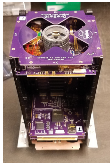
▲ The telescope peers out the end of OreSat, a two-unit CubeSat 10 × 10 × 20 centimeters on a side (about 4 × 4 × 8 inches). A 3D-printed protective shroud holds it in place.
