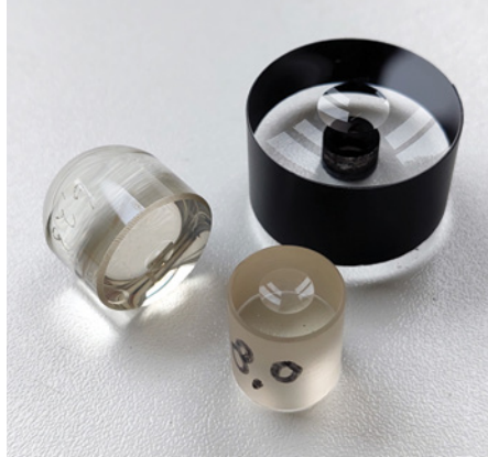
▲ A lens mold (bottom) inspired a rough prototype (left), which eventually led to the final concept (top right).
