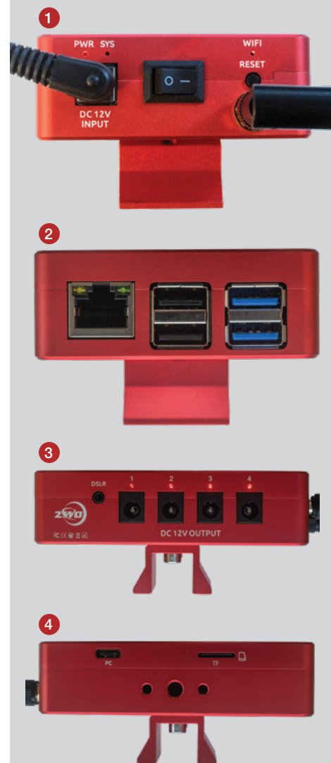
▲ As a control station, the ASlair Plus is loaded with ports and switches. ① This end includes the 12-volt, 5-amp power input, the on/off switch, and the Wi-Fi antenna at right along with the reset button and a red LED indicator. ② Four USB ports are located on the opposite end — two black USB 2.0 and a pair of blue USB 3.0 ports. An Ethernet port at left permits hardwiring of the device to a network. ③ A single jack at left connects to the shutter release cable of certain Canon or Nikon DSLRs. Four power ports line this side of the device, each having an LED indicator that lights up when each is activated in the ASlair app. ④ The side opposite of the power ports has a USB-C connection used to transfer files from the device's internal memory. The TF card slot (commonly known as a Micro-SD card) accepts up to 1-terabyte cards. At center is a 1/4-20 threaded hole for mounting the device. The smaller threaded holes are an alternative connecting location for the mounting shoe (seen at the bottom of the unit).
