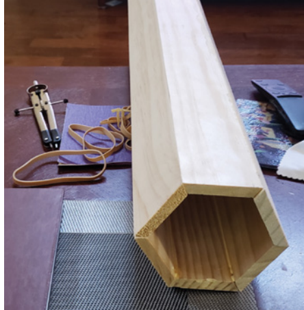
▲ The tube is assembled from straight boards beveled to 60° and arranged in a hexagon.
