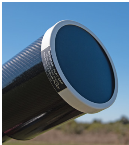
▲ Daystar offers an optional FlatCap diffuser that permits imagers to use the Sun as a light source for making flat-field calibration images to correct for uneven illumination and dust motes.
