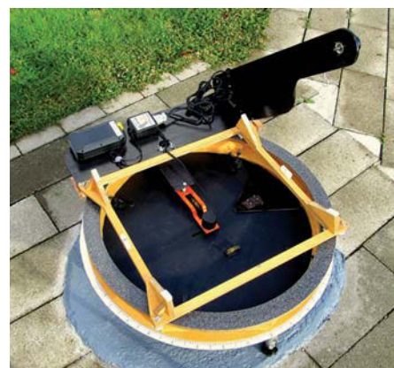
▲ The encoders are mounted at the ends of arms that reach from the telescope's framework to the center of rotation on the altitude and azimuth axes.
