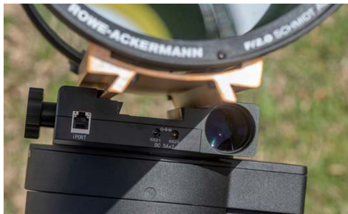
▲ Left: The CEM70G's 9½-kg counterweight can collide with the right ascension drive housing when balancing light loads; an optional smaller weight is recommended for such payloads. Right: The built-in iGuider is permanently installed within the saddle. Its objective is recessed about 50 mm inside the housing to prevent dew formation on the lens. A threaded aluminum cap covers the objective when not in use. Two slightly differing 12-volt DC power ports are seen to the left of the objective. The iPORT socket at left is used to connect other proprietary iOptron accessories.
