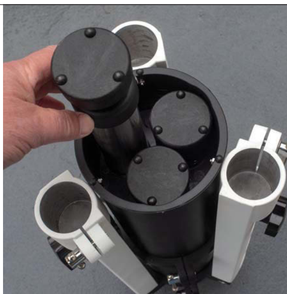
◀ Far left: The iOptron Tri-Pier's center column varies in height by sliding its center column up and down using indexed holes and spring-loaded bearings. Permanently installed anti-vibration pads on each foot ensure vibrations cease in a second or less.
