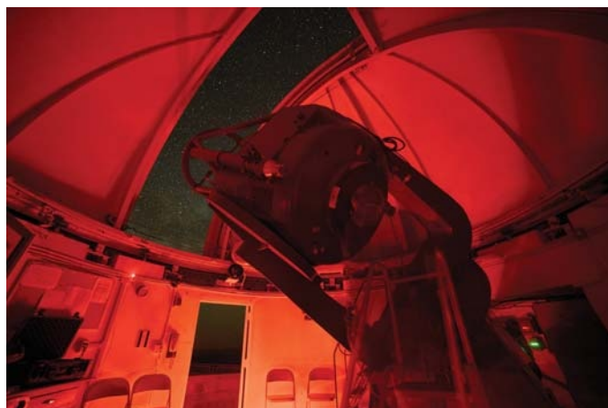
▲ REACHING OUT The 36-inch Dall-Kirkham reflector telescope at McDonald Observatory is used for public outreach programs, including the facility's Special Viewing Nights. Completed in 1956, the telescope was designed primarily for photometry.
