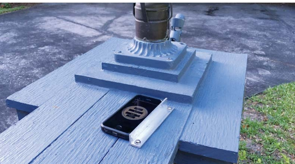
▲ Left: The bracket aligned to true north is fixed near Alberto Sagüés's observing spot, where he places his smartphone to record the direction to within half a degree. Right: He then transfers the reading to the telescope via an angle-measuring smartphone app.
