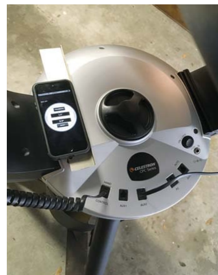
▲ Left: The bracket aligned to true north is fixed near Alberto Sagüés's observing spot, where he places his smartphone to record the direction to within half a degree. Right: He then transfers the reading to the telescope via an angle-measuring smartphone app.
