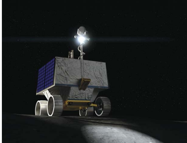
▲ ROVER INVESTIGATION NASA's Volatiles Investigating Polar Exploration Rover, or VIPER, is a mobile robot that will roam around the Moon's south pole looking for water ice using neutron spectroscopy.
