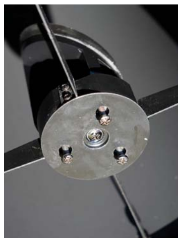
▲ The 2½-inch-wide secondary mirror assembly features a robust central hub that's slightly bigger than the width (minor axis) of the secondary mirror itself. Its three collimating screws make adjustments easy. The tube's interior is evenly painted flat black throughout.
