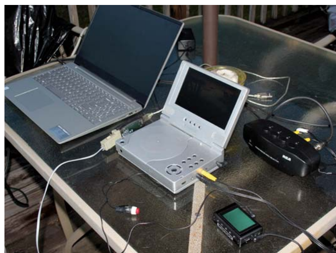
▲ OFF-SCOPE GEAR From left to right, the author's laptop computer, video display (a portable DVD player), and digital video recorder ready for an evening of fun. The cable switch box (far right) is used to send video output to either the display or the DVR.
