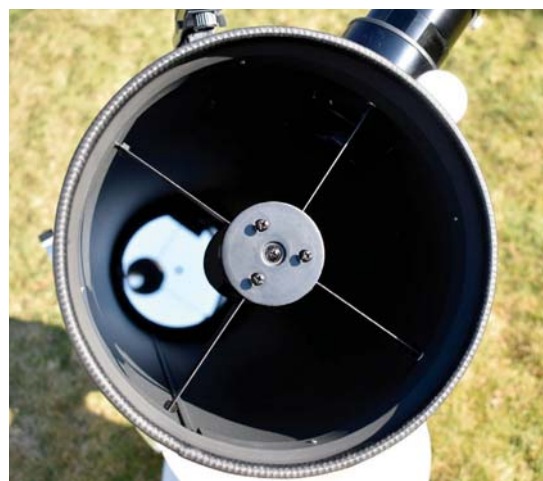
▲ The 2½-inch-wide secondary mirror assembly features a robust central hub that's slightly bigger than the width (minor axis) of the secondary mirror itself. Its three collimating screws make adjustments easy. The tube's interior is evenly painted flat black throughout.
