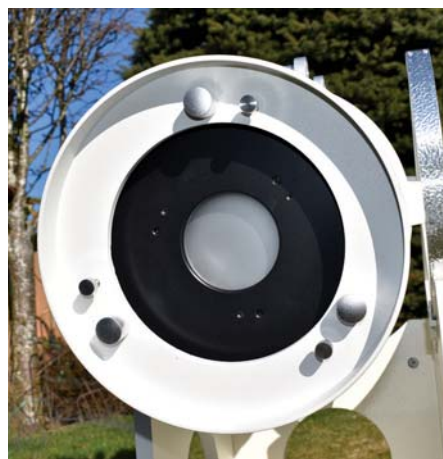
▲ The scope's mirror cell features three easily manageable collimating screws and three smaller locking screws. Note the textured metal surface on the altitude bearing (right), which permits smooth up-and-down motion.
