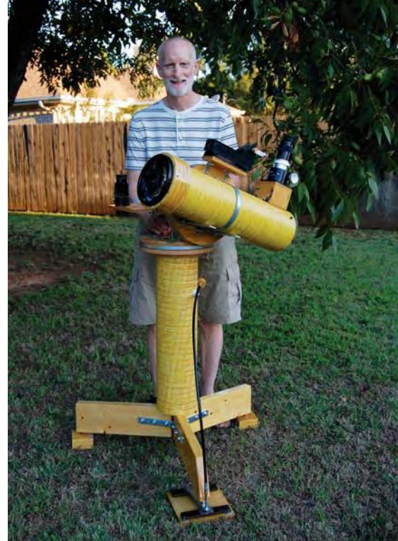
▲ Art Gamble's latest telescope uses a fiberglass tube and lazy Susan bearings to achieve a masterpiece of form and function.
