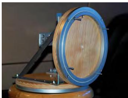
▲ The lazy Susan bearing surface is smooth aluminum with stainless steel rollers. No play or roughness here!
