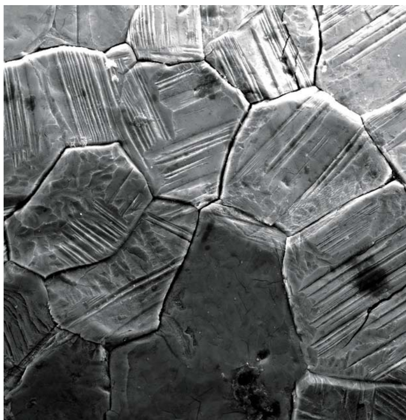
▲ CRYSTAL SURFACE This scanning electron microscope image, 80 microns to a side, shows the crystal structure on the surface of a micrometeorite. This meteorite is primarily made of iron, with small amounts of other elements. Iron micrometeorites are easy to find with the help of a strong magnet.
