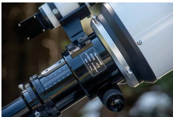
▲ Left: The telescope's solid 3.4-inch rack-and-pinion focuser and mounted 8x50 right-angle finderscope are rotatable by loosening the large metallic "captain's wheel" ring with machined spokes. Right: A millimeter scale to aid in repeating focus positions is printed on the focuser drawtube. Also visible is the 10:1 fine-focus knob.
