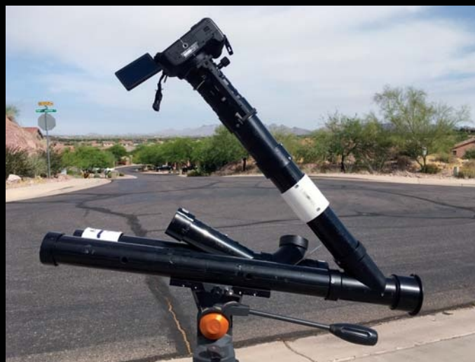
▲ Joseph Gerencher's spectrograph uses a traditional slit but a decidedly non-traditional CD or DVD for a diffraction grating. Light enters on the left, bounces off the grating at the junction on the right, and goes through a lens at the white coupling partway up. The resulting spectrum reaches the camera body (without lens) on top.
