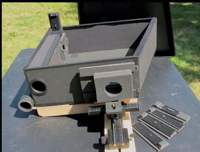
▲ David Britz's spectrograph uses a polished metal rod in place of the more traditional slit. Light enters on the left, bounces off the rod in back, and illuminates the diffraction grating in front right. The camera (not mounted here) slides left and right to capture the entire spectrum. Different diameter rods, visible on the right, provide different resolutions.
