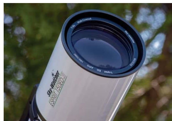
▲ The telescope's 150-mm f/7 (1,050-mm focal length) air-spaced, three-element objective incorporates one element made with FPL-53 extra-low-dispersion glass and two BK7 elements. Its retractable dewshield is secured with two thumbscrews.
