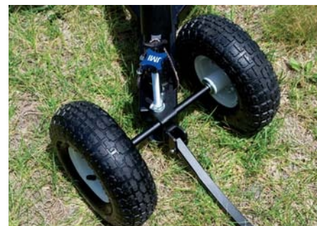
▲ The steering wheels have a limited turning range due to the 10-inch pneumatic tires hitting the north foot plate of the Wheeley Bar assembly, resulting in a wide turning radius.
