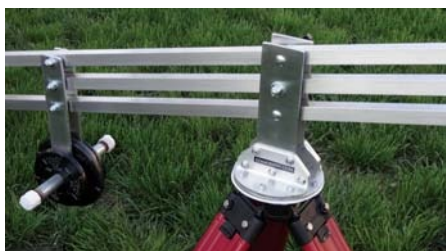
▲ Top: Photographers' pistol-grip ball-heads allow for easy aiming of the binoculars. Bottom: The heavy-duty central pivot is key to the Binocrane's success.
