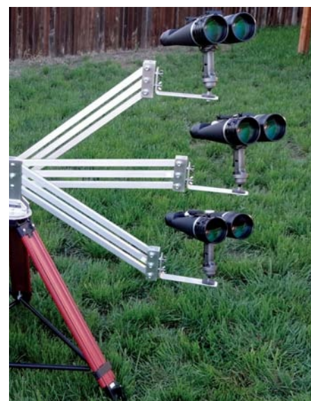
▲ The ends of a parallelogram remain parallel when the arms are raised or lowered.
