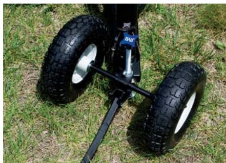
▲ The steering wheels have a limited turning range due to the 10-inch pneumatic tires hitting the north foot plate of the Wheeley Bar assembly, resulting in a wide turning radius.
