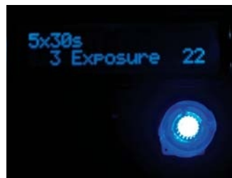
▲ The controller's display lets you know what it's doing at the moment, as does the knob's color. In this example it's taking five 30-second exposures, it's on exposure number three with 22 seconds left, and the blue knob indicates that the shutter is open.
