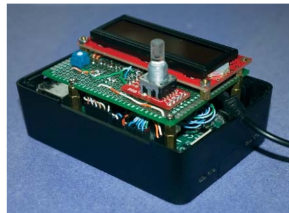
▼ The Raspberry Pi and custom control circuit fit in a small project box.
