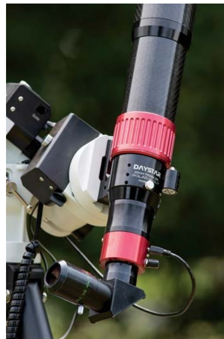
▲ The mounting shoe on the SS60C is threaded to attach to most photo tripods, and its base is formatted to fit in any Vixen-style dovetail saddles. Users need to supply their own star diagonal and eyepieces.
