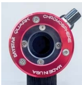
▲ The exit aperture of the Quark filter is large enough to display the entire solar disk using a 40-mm Tele Vue Plössl.
