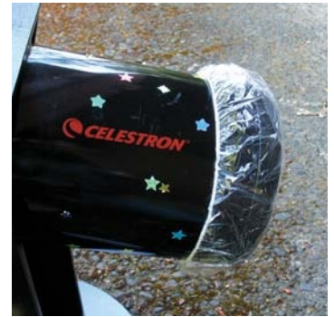
▲ CELL PROTECTION A simple shower cap prevents dust from entering through the bottom of the telescope around its mirror cell.
