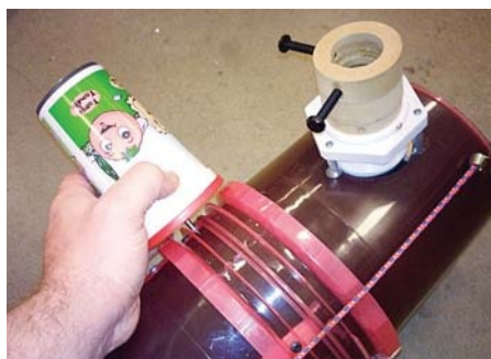
▲ Brent screws on one of the altitude bearings. The 1¼-inch helical focuser is made from a plastic toilet valve.
