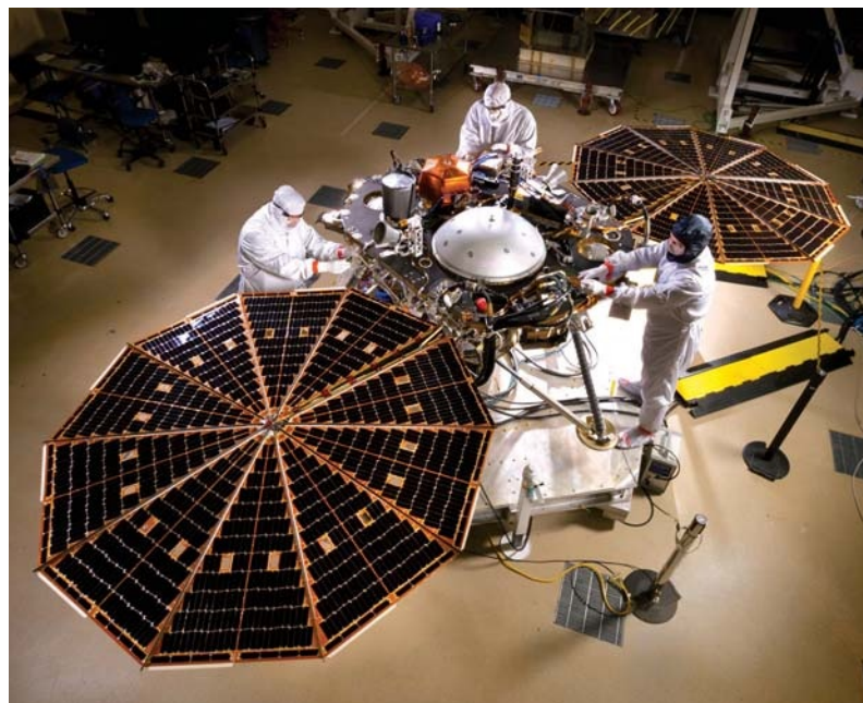
▲ PROVEN DESIGN Shown during testing in 2015, Insight inherited its structure and many of its components from the Phoenix lander, which Lockheed Martin likewise built for NASA.
