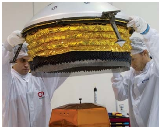
▲ NOISE-CANCELING DOME This tent-like shield will ensure that Insight's SEIS instrument (seen at bottom) is protected from seismic "noise" generated by Martian winds and wide temperature fluctuations.
