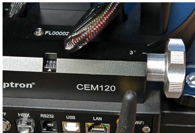
▲ Even with the CEM120 fully loaded with the telescope and 66 pounds of counterweights, the mount's calibrated azimuth (left) and altitude (right) controls worked very smoothly for polar aligning the mount.
