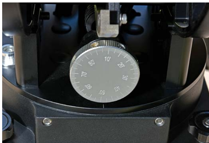
▲ Even with the CEM120 fully loaded with the telescope and 66 pounds of counterweights, the mount's calibrated azimuth (left) and altitude (right) controls worked very smoothly for polar aligning the mount.
