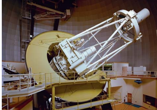
▲ GOOD OLD DAYS Left: David Malin is seen in the prime focus cage of the 4-meter f/3.3 Anglo-Australian Telescope. Right: The AAT with its massive horseshoe equatorial mount.
