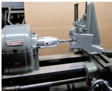
▲ Bob made a sphere-cutting tool for his lathe so he could make the inner planets himself.
