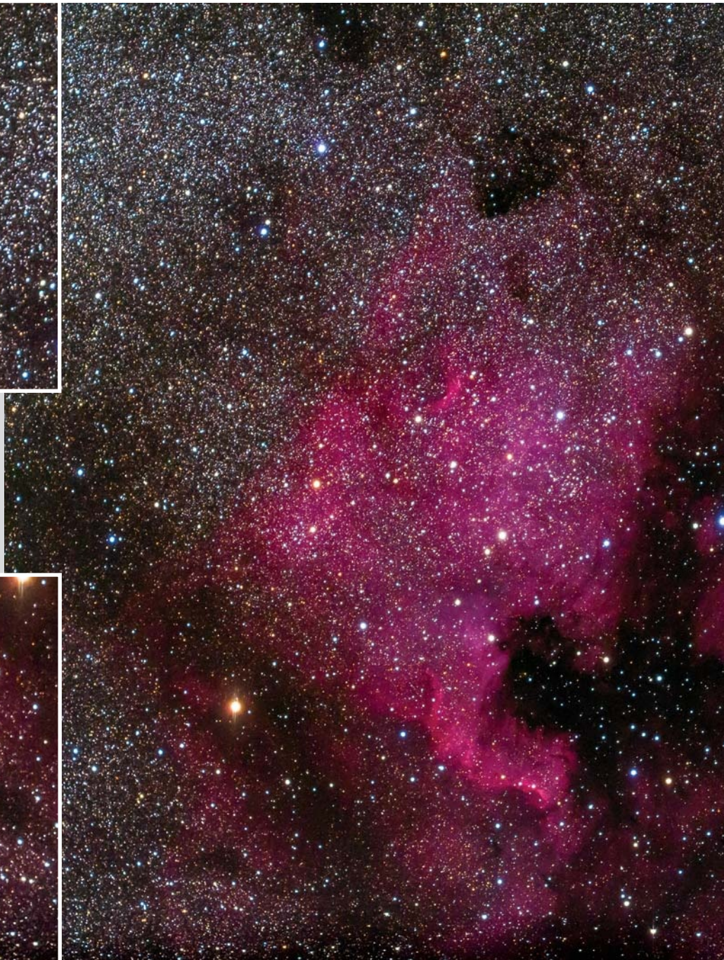
A single 5-minute exposure with a modified Canon 5D MkII DSLR at ISO 1600 shows stars as pinpoints to the very corners of the full-frame sensor (insets). Focus was uniform across the field. The slight asymmetric purple halo around Deneb is an artifact from the camera's internal IR filter and is seen in images taken with all telescopes.
