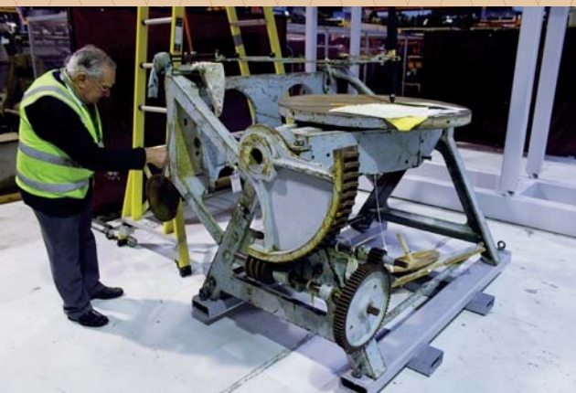
▲ THE GREAT GRINDER While most ASV volunteers focused on the telescope itself, the oldest ASV team member, David Linke, devoted his attention exclusively to Thomas Grubb's two-ton mirror-grinding and polishing machine. The apparatus was used several times in the 19th century to remove tarnish that gradually accumulated on the GMT's speculum mirrors.
