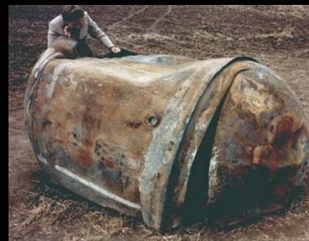
▲ LONE STAR The main propellant tank of the second stage of a Delta 2 launch vehicle landed near Georgetown, Texas, on January 22, 1997. The approximately 250-kg tank is primarily made of stainless steel and survived reentry relatively intact.
