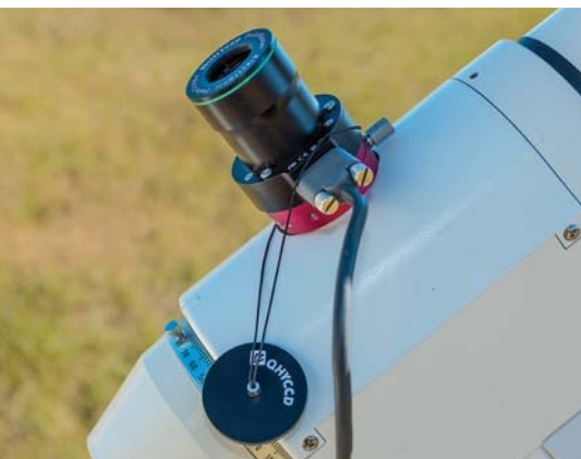
▼ Left: Using one of the well-machined adapters offered for popular mounts, the PoleMaster clamps over the polar-scope aperture of a German equatorial mount. Middle: When the PoleMaster is not in place, the aperture remains open to allow using the polar-alignment scope as usual, which is often necessary for the initial rough alignment. Right: When not in use at all, a supplied metal cover clamps over the adapter, to prevent dust from entering the polar axis. The camera also includes a screw-on metal cover.
