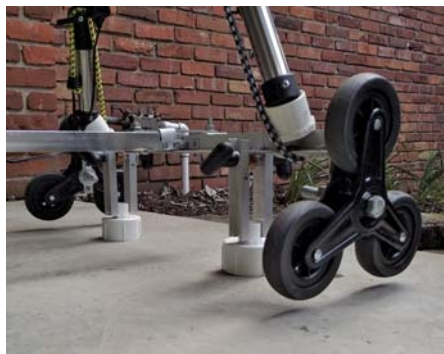
▲ Stabilizing legs swing down to lock the platform in place when observing.
