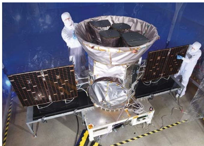
▲ DETAIL WORK Visible in this lab shot are TESS's four cameras (top), which appear to sit like eggs inside the nest of the sunshield.
