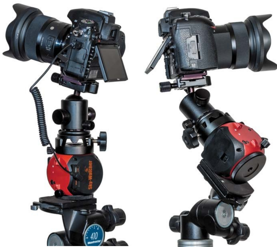
▲ Left: When mounted for time-lapse shooting, the drive remains balanced over the tripod, and can now turn in azimuth for panning along the horizon. Here, SAM is mounted to a standard tripod head. While the adapter plate is supplied, users must supply their own ball head. Right: For sequences in its unique “Astro Time-Lapse” mode, SAM must be set up as a polar-aligned tracker, but with the camera now framing a horizon scene, for tracked time-lapses of the moving Milky Way or bright comet over a fixed landscape.
