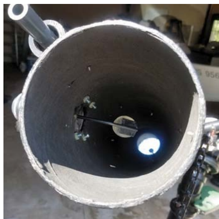
The secondary mirror is mounted on a single arm that allows it to swing sideways and move in and out. Note the pipe used as a finder.
