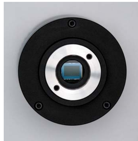
▲ The camera features a 2.3-megapixel Sony IMX302 CMOS sensor, seated just behind the C-thread housing. Users may need to provide their own C-to-T-thread adapter to attach the camera to some telescopes and accessories.
