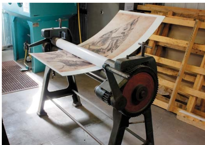
▲ SHAPING THE ROOF Each section of the dome roof was bent into shape using a large slip roller.
