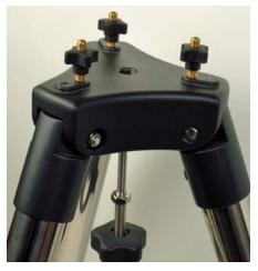
Orientation of the saddle plate is important for the mount's level-and-go setup. Your telescope's aperture must point in the direction of the small white triangle on the plate. Above: Attaching the AZ Mount Pro to the 2-inch tripod requires first installing three leveling knobs within the inner set of threaded holes.
