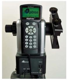
▲ iOptron's Go2Nova 8407 controller includes a database of more than 212,000 objects, including the Messier, NGC, and IC catalogs, as well as many solar system objects (though excluding Pluto). A bracket is included on the mount to conveniently hang the hand paddle when not in use.
