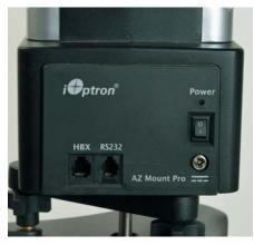
▲ There are three input ports on the base of the mount. The HBX port accepts the Go2Nova hand controller, while the RS232 serial port is used to connect to a computer, though you'll need to provide your own serial-to-USB adapter if your computer lacks a serial port. The port at right is for the AC charger.
