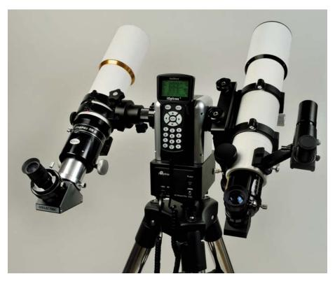
▲ An optional Vixen-style saddle (\$79) is available that replaces the counterweight, permitting users to mount a second telescope.
