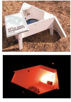
▲ Corner gussets and slightly angled legs provide stability. Angle aluminum edging keeps the lid from sliding off.
