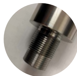
◀ The counterweight shaft includes a section of lead-in threads designed to lessen the chance of cross-threading when attaching to the mount.
