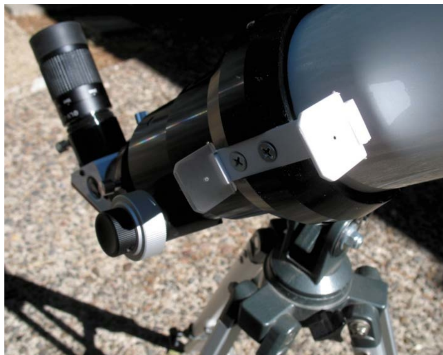
▲ This folding finder casts a bright spot on a frosted screen. The front element shades the screen, and sunlight shines through the hole.
