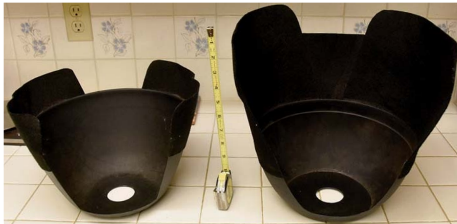
▲ Make a generous cutout in the side of the bowl that will face the ground, and add felt wings if necessary to block light from the sides.
