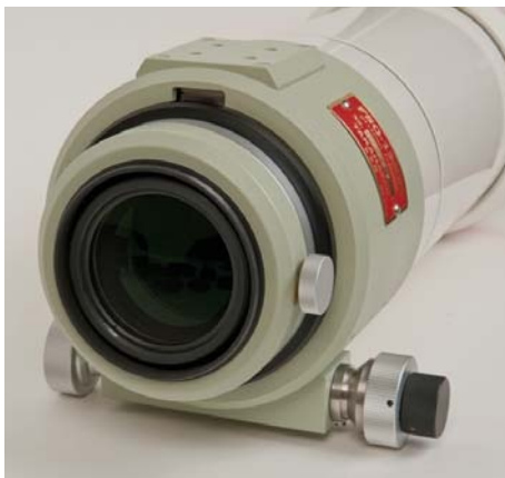
▲ The telescope's 3-element objective and 2-element rear corrector include three lenses made from “super” extra-low-dispersion glass.
