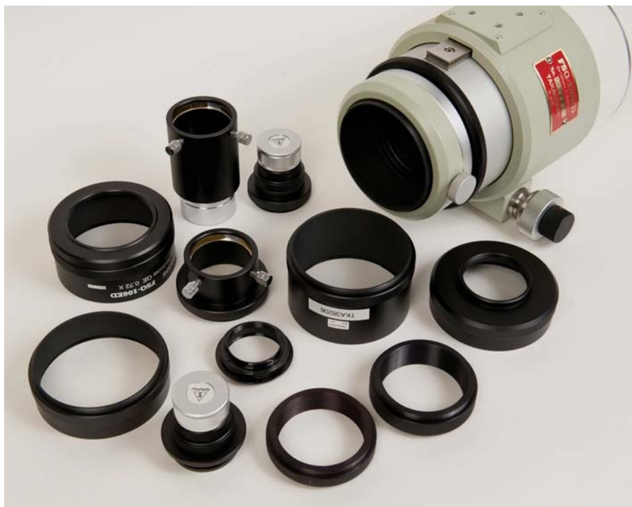
▲ This collection of adapters (with several comprising two pieces already screwed together) is what the author needed to use the FSQ-130ED with 1¼- and 2-inch eyepieces, with his Nikon DSLR camera, and with Apogee and FLI large-format astronomical CCD cameras.
