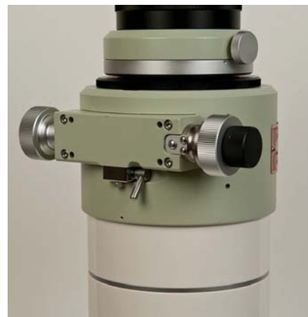
▲ As described in the accompanying text, an adjustable-friction locking lever on the focuser prevents the drawtube from slipping while still allowing focusing with the coarse and 10:1 fine-focus knobs.
