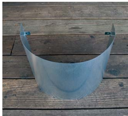
▲ Left: Replace the carriage light with a downward-facing fixture and a downward-facing flood bulb. Note the brackets for mounting the shield that are attached to the siding. Middle: Install the brackets on the wall, and then attach the shield (shown assembled). Right: The finished shielded fixture casts its light downward where it's useful, not outward into your eyepiece.
