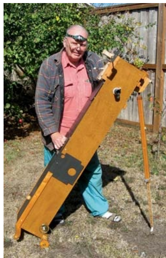
▲ Above: Craig Daniels with his Dogson telescope. Right: The top end of the Dogson holds the eyepiece, setting circles, split-pupil finder, and swing-out camera mount.
