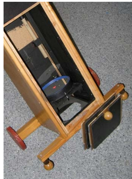
▲ The inside of the Dogson, showing the primary mirror sled.
