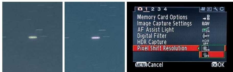
▲ The K-3 II's Pixel Shift mode moves the sensor by one pixel over four exposures to improve resolution and reduce noise in exposures 30 seconds and shorter. However, moving targets such as stars can exhibit pixelated artifacts in RAW files, either when developed in Adobe Camera Raw (left), and to lesser extent even in Ricoh's own RAW developing software Digital Camera Utility that comes with the camera (middle).
