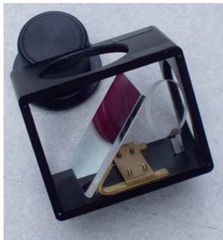
The flip mirror housing with the cold mirror and corrector plate installed.
