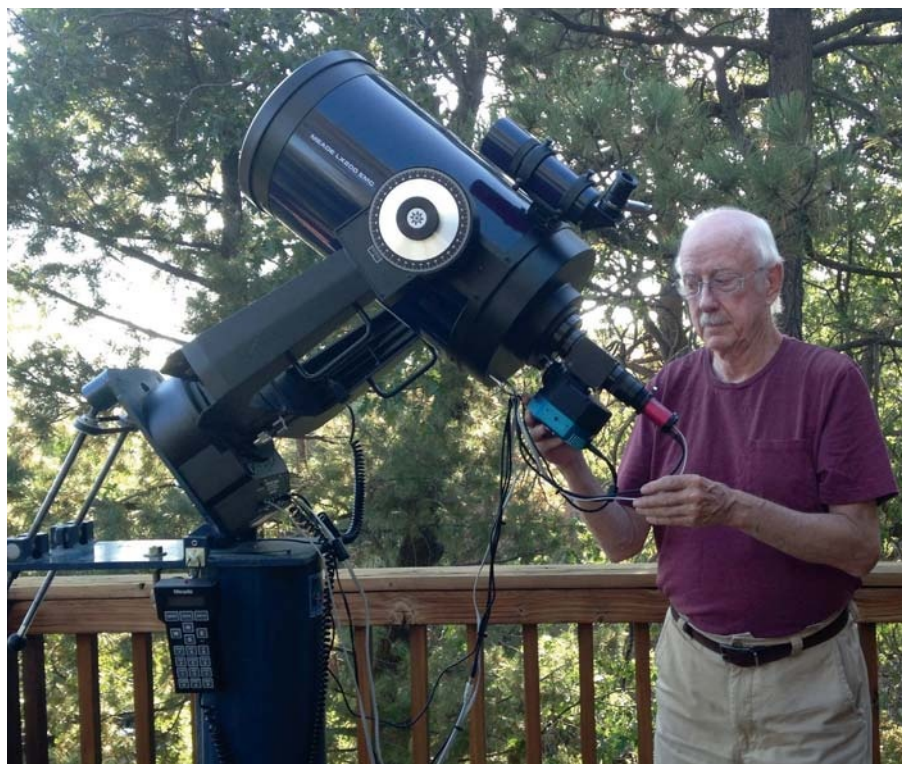
▲ Don Rea with his fully assembled telescope and guide setup. The imaging camera is on the bottom, with the guide camera to the right.
