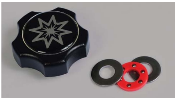
A milk-jug washer next to the altitude locking knob reduces but does not eliminate the knob's tendency to bind. A better fix is to order an inexpensive three-piece thrust ball bearing from McMaster Carr ( mcmaster.com ).
