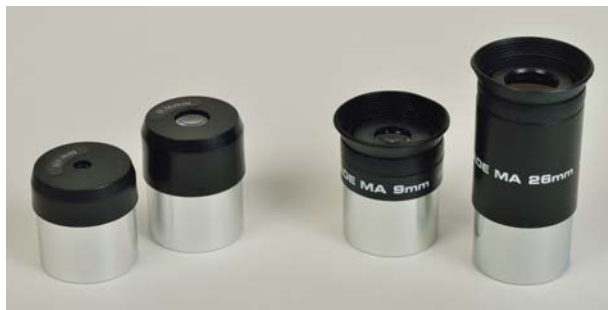
Baby's Huygenian eyepieces at left look very much like Mama's and Papa's modified achromats, but the modified achromats have much better optical quality.
