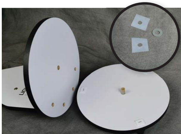
Above: Inspect the Teflon pads on the base. Smooth off any rough spots and countersink any staple that protrudes above the pad. Inset: Cut the two "washers" shown here from the sides of a plastic milk jug, sandwich a USS \frac{1}{2} -inch washer between them, and stack them on the spindle. (The steel washer has a \frac{5}{16} -inch inner diameter and 1\frac{1}{8} -inch outer diameter.) When re-assembling the mount, tighten the lock washer and then back it off about \frac{1}{4} turn to make sure that the turntable rotates smoothly.
