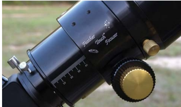
The imaging version of the SVA-130T includes a heavy-duty, 3-inch Feather Touch focuser. This dual-speed focuser can be rotated 360^\circ and is locked in place with three knurled brass knobs spaced at 120^\circ intervals around its base.
