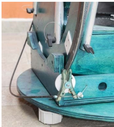
The clamp came from a battery charger, and the rotor is made from sheet metal.
