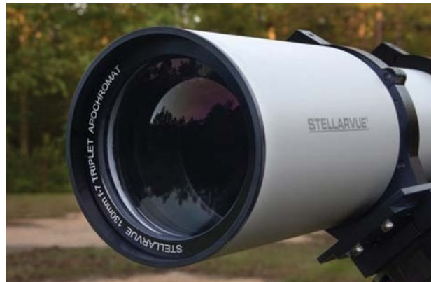
The scope's objective is an air-spaced triplet made with a super-low-dispersion ED glass center element and a Lanthanum rare-earth rear element.
