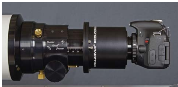
The focal reducer/field flattener attaches to the Feather Touch 3-inch focuser using a custom adapter that also includes collimation adjustments, though the unit is collimated at the factory.
