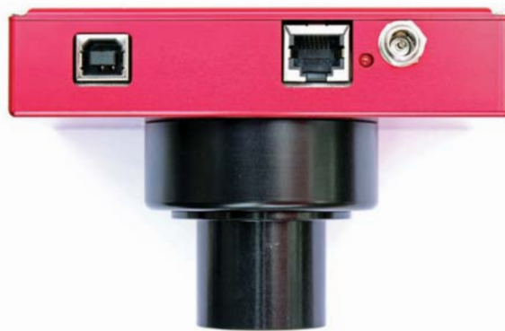
Left: The Infinity's \frac{1}{2} -inch format Sony ICX825 EXview HAD CCD II detector boasts high quantum efficiency, meaning you'll record faint objects with fairly short exposures. Right: Three ports on the bottom of the Infinity are a B-type USB 2.0, an RJ-12 port that allows the camera to be used as an autoguider, and a DC power input. The red LED is activated only when the camera is connected to your telescope mount.
