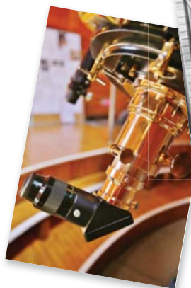
Left: The brass sections of the refractor, including the eyepiece assembly, were disassembled, cleaned, repaired, clear-coated, polished, and reassembled.
