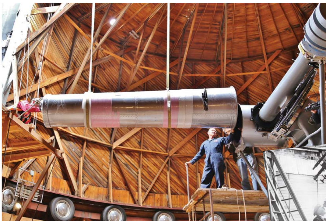
Left: Lowell Observatory's Director of Technical Services, Ralph Nye, supervises the reinstallation of the rear tube section of the Clark telescope during its renovation.
