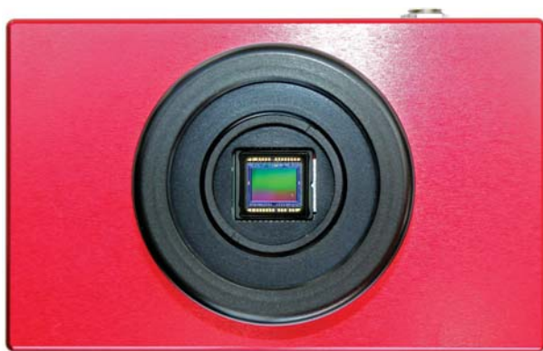
Left: The Infinity's \frac{1}{2} -inch format Sony ICX825 EXview HAD CCD II detector boasts high quantum efficiency, meaning you'll record faint objects with fairly short exposures. Right: Three ports on the bottom of the Infinity are a B-type USB 2.0, an RJ-12 port that allows the camera to be used as an autoguider, and a DC power input. The red LED is activated only when the camera is connected to your telescope mount.
