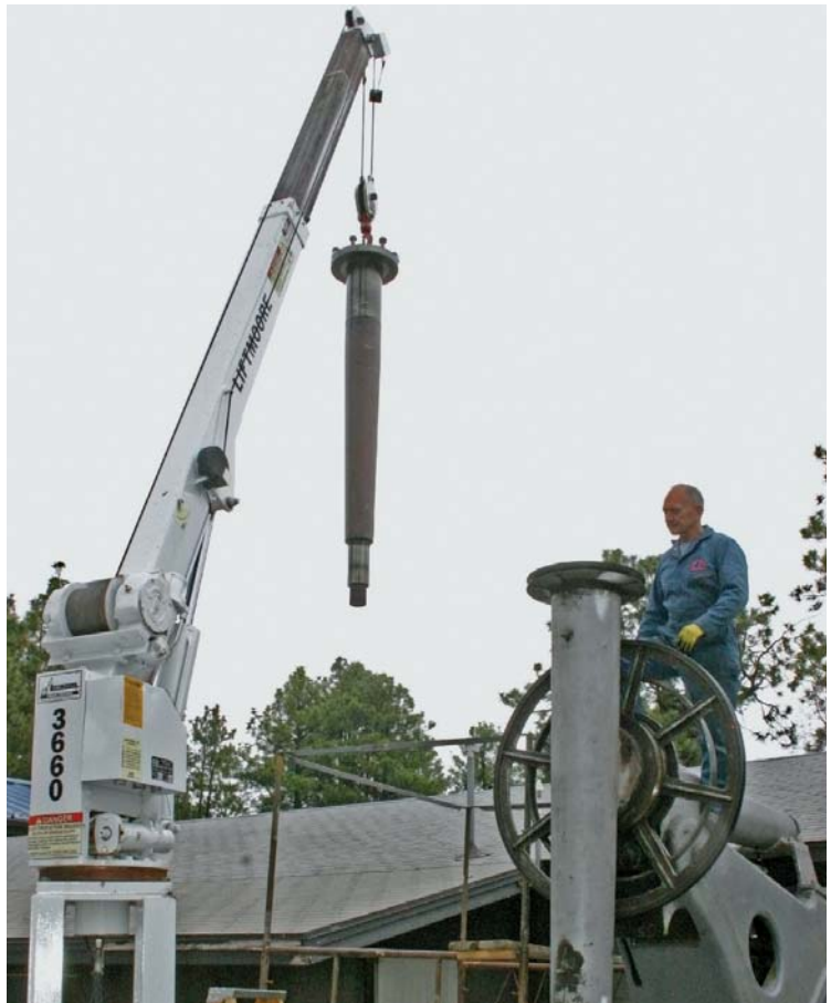
DISASSEMBLY A crane lifts the 900-pound declination shaft out of its housing for inspection and cleaning. The mount was bolted to a temporary pier at a 35° angle, so the polar axis (behind the big right-ascension circle) would be horizontal for easier removal of parts.
