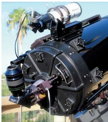
Adding 10 cooling fans to this 14-inch telescope yielded a dramatic improvement in steadying the view.
