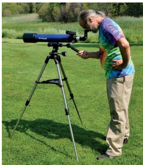
Left: The Infinity 90 includes a quality image-erecting prism that makes the scope useful for both terrestrial and astronomical observing. Middle: Even when fully extended, the Infinity 90 tripod is short. While this provides a stable view at high magnification, a low stool or observing chair is required for comfortable viewing in most positions. Right: Aiming the refractor at targets anywhere near the zenith is awkward, due to the position of the red-dot pointer. A better placement for the finder would be near the objective lens.
