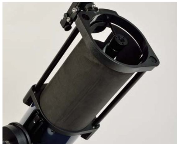
The OneSky's collapsible tube is susceptible to stray light that can compromise its otherwise excellent views. The author made this simple shroud out of a piece of lightweight foam that can be found at most arts and crafts stores.
