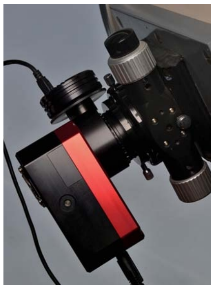
Bottom: Even with its off-axis guider and internal filter wheel, the Atik One takes up very little focus travel (requiring a total of 47 mm of additional focus travel), allowing it to be used with fast Newtonian reflectors such as the author's 12½-inch f/4 with a Baader coma corrector.
