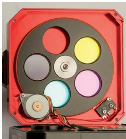
Left: The camera housing contains a slim, internal filter wheel that accepts standard 1¼-inch color filters (not included), though the camera does not incorporate an internal shutter. Users may want to consider filling the 5 th filter slot with an opaque filter to use when recording dark and bias calibration frames.
