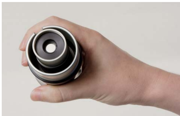
Top: The Quark's 1¼-inch nosepiece houses a 12.5-mm blocking filter that reduces the light entering the etalon to safe levels. Because the telescope's light path is converging, this filter doesn't constrict the light path at all. Above: the final 21-mm filter before the eyepiece provides an evenly illuminated view of the solar chromosphere. The 1¼-inch eyepiece holder is upgradable to a 2-inch version.
