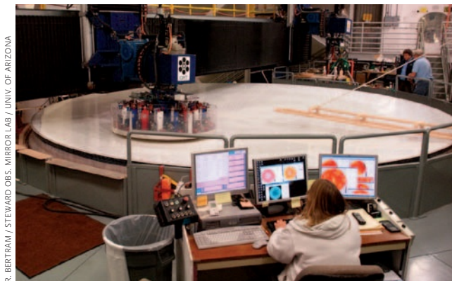
POLISHING An engineer monitors the Large Polishing Machine as it shapes the first GMT mirror. Tests are performed throughout polishing to ensure the mirror's face has the correct shape.
