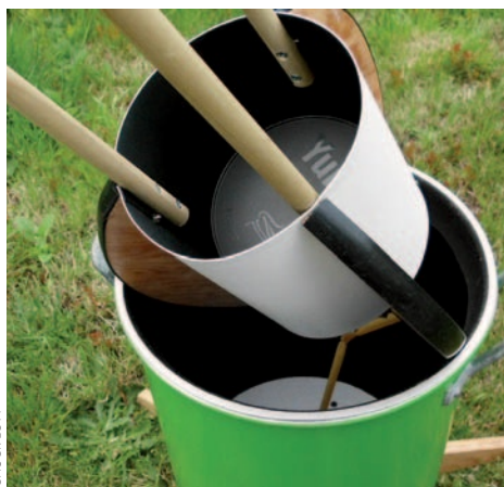
A length of surgical tubing serves as a spring to prevent the scope from nosediving when aimed near the horizon.
