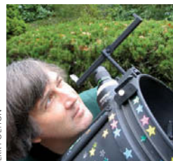
Jerry Olton is shown using his “split-pupil” finder. He notes that it’s best to position your eye just behind the lens and look over the top of it to see the sky and pointer arrow sharply focused.
