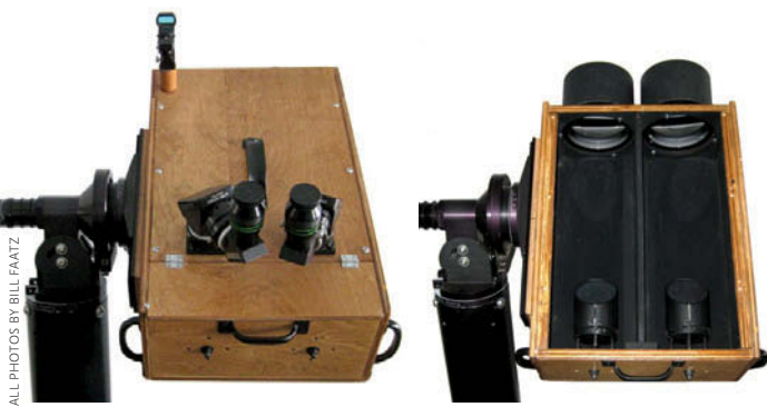
Each half of the binocular uses a pair of star diagonals — a 2-inch model and a 1¼-inch that holds the eyepieces. Inter-ocular spacing and rough focusing is done with helical focusers, while fine focus is achieved by sliding the eyepieces in and out of the star diagonals.
