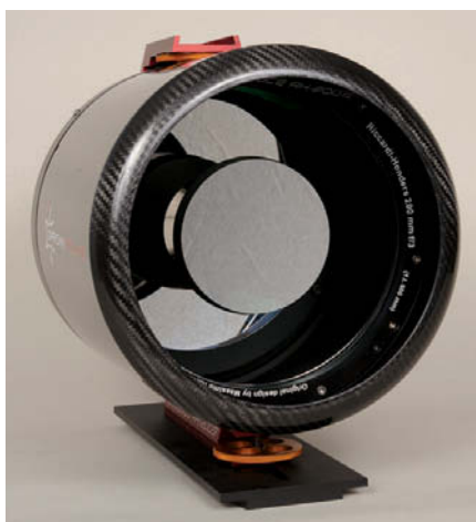
Left: As explained in the text, full-frame DSLR cameras work best when used with special adapter rings. Center: The Riccardi-Honders optical design in the RH200 has a full-aperture corrector with an aluminized spot on its back side forming the Cassegrain secondary mirror. Right: Some camera setups have limited clearance with the optional RoboFocus system (see the accompanying text for details).
