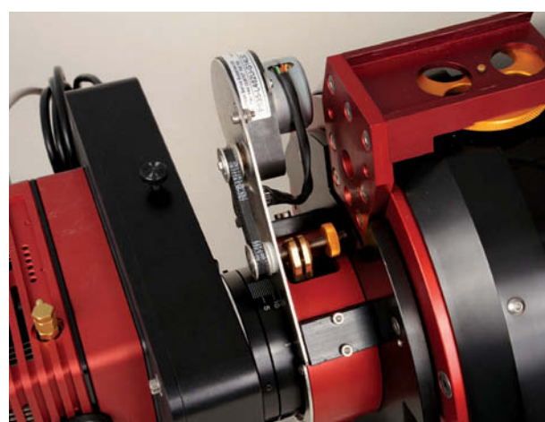
Left: As explained in the text, full-frame DSLR cameras work best when used with special adapter rings. Center: The Riccardi-Honders optical design in the RH200 has a full-aperture corrector with an aluminized spot on its back side forming the Cassegrain secondary mirror. Right: Some camera setups have limited clearance with the optional RoboFocus system (see the accompanying text for details).
