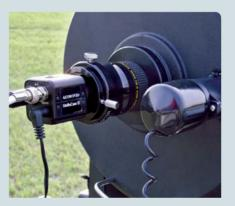
Observing with an astrovideo camera like the one here doesn't require much additional equipment to tow into the field. Besides the camera, you'll need a DC power source and a video monitor or laptop computer to display your exposures. You can also use a variety of Barlows and focal reducers to tailor your field of view to each target, just like switching eyepieces when visually observing.
