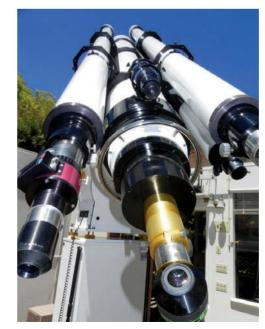
The business end of the 12-inch refractor includes a very large stainlesssteel "yacht steering wheel" made by Ed Byers. It allows the observer a convenient handhold for swinging the big telescope and its auxiliary instruments around the sky.
