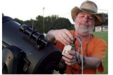
Left: Setting up an astrovideo camera couldn't be easier — simply replace your eyepiece with your astrovideo camera. Your telescope then becomes the camera's lens.
