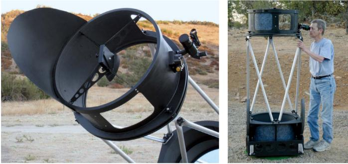
Tilting the focuser back toward the primary mirror by 11° relative to the primary's optical axis allowed Highe to shave 4 inches off the eyepiece height when the scope is aimed at the zenith. The spider assembly for the scope's secondary mirror, like the support system for the primary, is a significant departure from traditional designs. Its construction is also carefully described in his book, which includes software and Excel worksheets for modifying the design for other telescopes.
