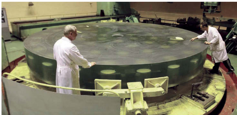
Opticians prepare to remove the topmost 8 mm of glass — and with it a host of imperfections — from the original 6-meter primary mirror for Russia's Bolshoi Teleskop Azimutal'ny.
