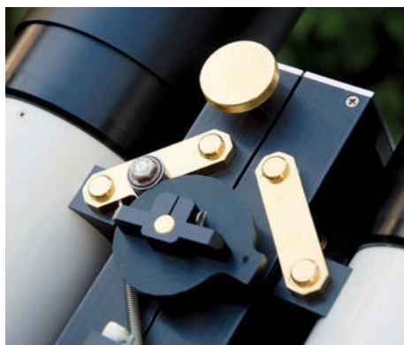
Left: Each binocular half features a Crayford focuser and a housing that holds two diagonal mirrors feeding light to the eyepiece and providing a right-reading view. Right: The adjustments that align the two optical tubes are crucial to the performance of a binocular telescope. The large black knob controls the intra-ocular spacing, while the gold-plated brass knob governs the vertical alignment.
