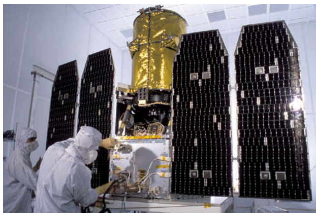
Technicians at Orbital Sciences Corporation test the solar arrays on the 620-pound (281-kg) spacecraft. GALEX is one of the smallest space telescopes launched by NASA in recent years.
