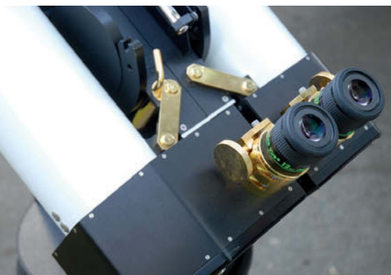
Left: Each binocular half features a Crayford focuser and a housing that holds two diagonal mirrors feeding light to the eyepiece and providing a right-reading view. Right: The adjustments that align the two optical tubes are crucial to the performance of a binocular telescope. The large black knob controls the intra-ocular spacing, while the gold-plated brass knob governs the vertical alignment.
